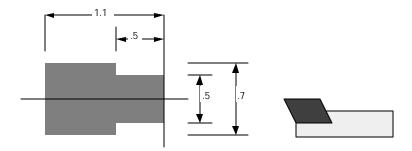
The next diagram shows the rapid moves as a lighter line, feed moves are shown as the heavier lines.
