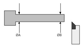
With this shaft,  $\emptyset A = \emptyset B$ . In order to do this, put an offset command at the end of the turn.
