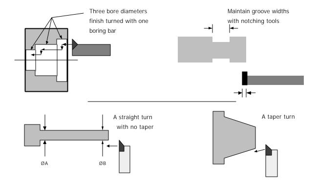
In all three cases it would be very advantageous to be able to have the operator make corrections to the parts that entail more than just moving the tool by changing the tool offset (T). If you made a change to the tool offset, the overall size of the part would change in each of the above examples.
