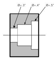
For this example, three diameters have to be turned with only one tool. Each of the diameters can have an individual offset.
