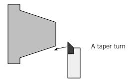
The actual taper that a tool cuts will depend on the toolnose radius. If this is not an easy tool to maintain then the taper will vary as the tool changes. Normally this would be a big problem. However with the secondary offsets this is very simple. We could put a secondary offset at the end of the taper and then turn the offset off. This would look like:
