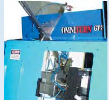
Simple track loader with in feed bin
