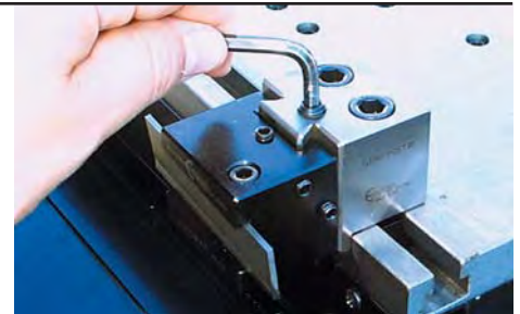
THE LOCKING WEDGE IS DRIVEN BY A SCREW FROM ABOVE
