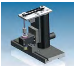
(Guards removed for picture) Vertical Setup Coarse and fine adjustments for cutter height
