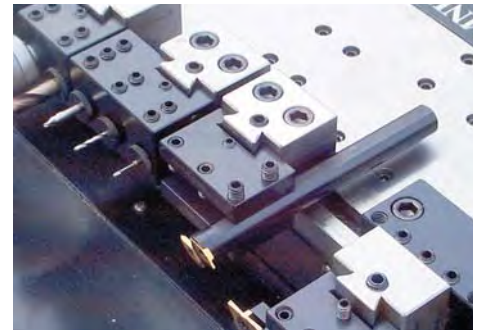
HOLDERS PLACED NEXT TO ONE ANOTHER WITHOUT INTERFERENCE
