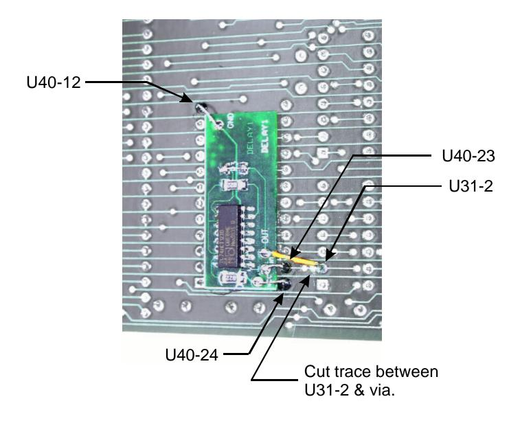
MC2 "Delay Board": Mounts on non-component side of MC2 opposite U40.
