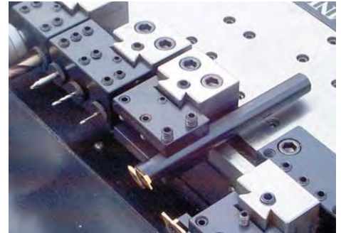
HOLDERS PLACED NEXT TO ONE ANOTHER WITHOUT INTERFERENCE
